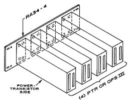
FIG. 1 MODEL RA 35-1 RACK ADAPTER.
