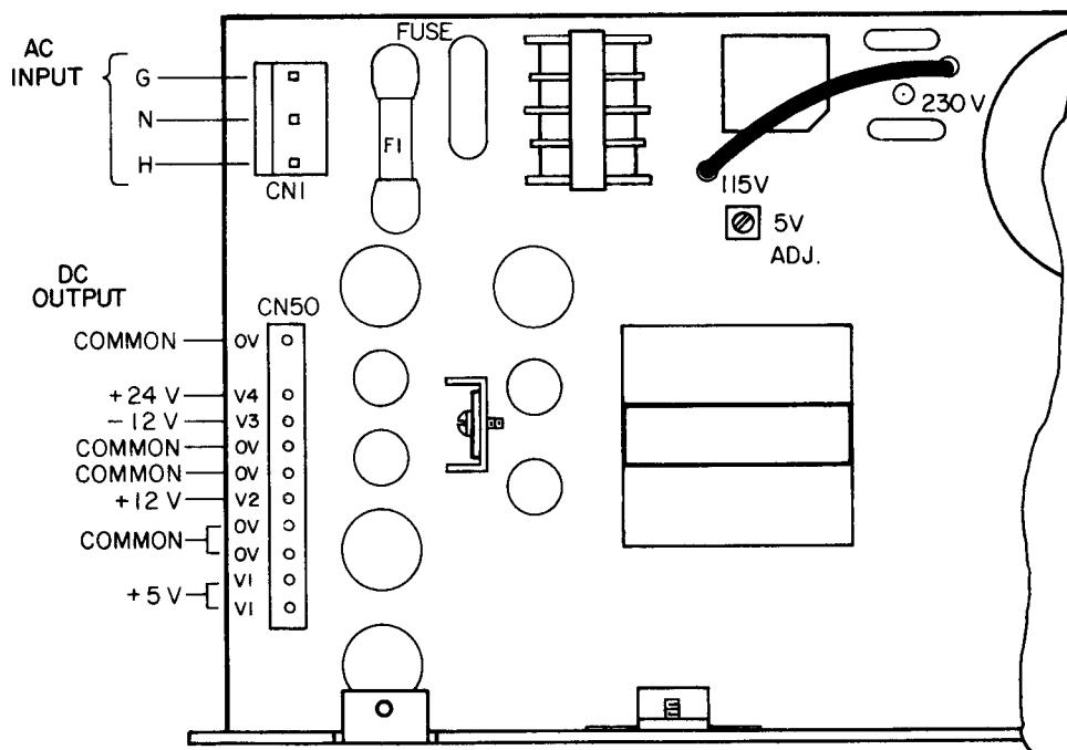
FIG. 1 SIMPLIFIED TOP VIEW, MODEL EMR 500K POWER SUPPLY.
