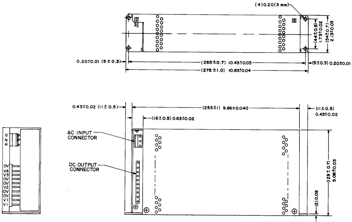
FIG. 2 MECHANICAL OUTLINE DRAWING, MODEL EMR 500K.
