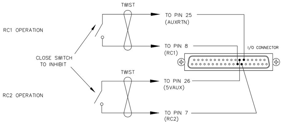
NOTE: AS AN ALTERNATIVE TO THE ABOVE CONFIGURATION, A HIGH LOGIC LEVEL CAN BE USED TO DRIVE RC2 AS LONG AS THE RETURN FROM THE EXTERNAL POWER SUPPLY IS CONNECTED TO AUXRTN. IN EITHER CASE, SWITCH CAN BE A RELAY CONTACT, LOGIC GATE, TRANSISTOR, ETC., OPERATED FROM, OR REFERENCED TO, THE 5VAUX SUPPLY.
