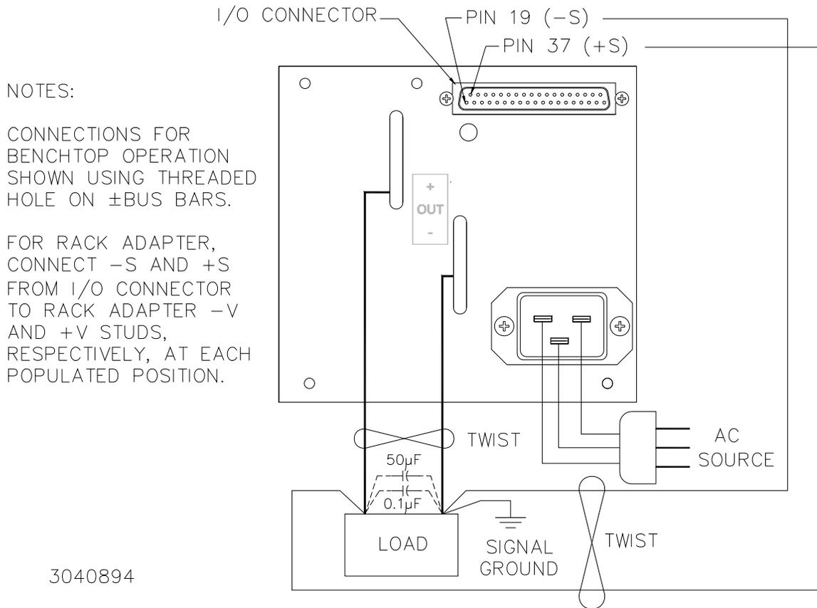
FIGURE 2-5. LOAD CONNECTION - METHOD II (REMOTE ERROR SENSING)
