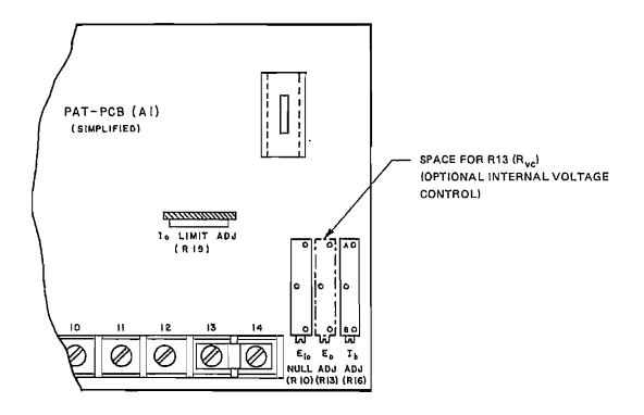
FIG. 5-2 INSTALLATION OF OPTIONAL CONTROLS.
