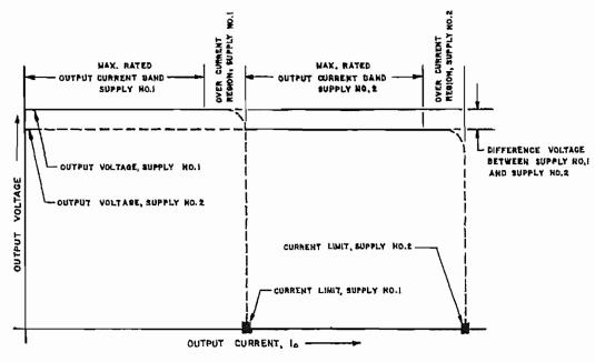
FIG. 3-12 PARALLEL OPERATION, PAT SUPPLIES.
