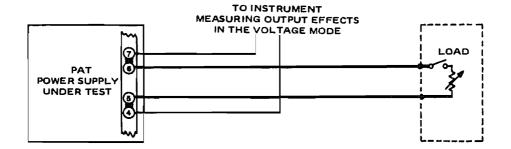
A) OUTPUT EFFECT MEASUREMENT (VOLTAGE) WITHOUT ERROR SENSING AT THE LOAD.
