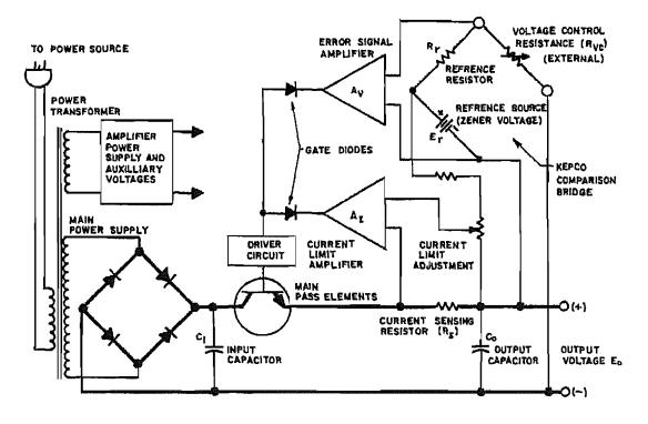
FIG. 4-1 SIMPLIFIED DIAGRAM, PAT POWER SUPPLIES.
