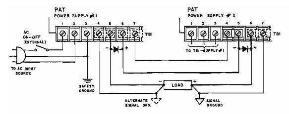
FIG. 3-11 SERIES CONNECTION OF PAT SUPPLIES.
