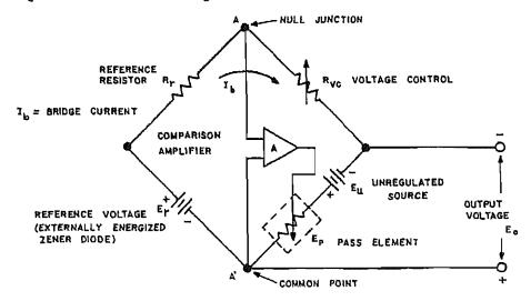
FIG. 3-4 KEPCO POWER SUPPLY AND COMPARISON BRIDGE CIRCUIT.
