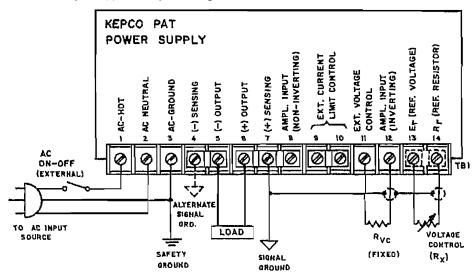
FIG. 3-9 CONNECTIONS FOR CONDUCTANCE PROGRAMMING.
