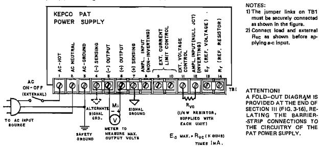
FIG. 2-4 OPERATIONAL CHECKOUT.
