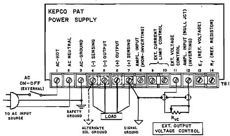
FIG. 3-2 LOAD CONNECTION WITH REMOTE ERROR SENSING.
