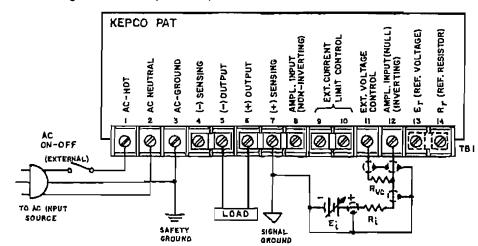
FIG. 3-10 CONNECTIONS FOR VOLTAGE PROGRAMMING.
