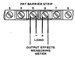
FIG. 5-4 APPROXIMATION OF A 4-TERMINAL NETWORK.
