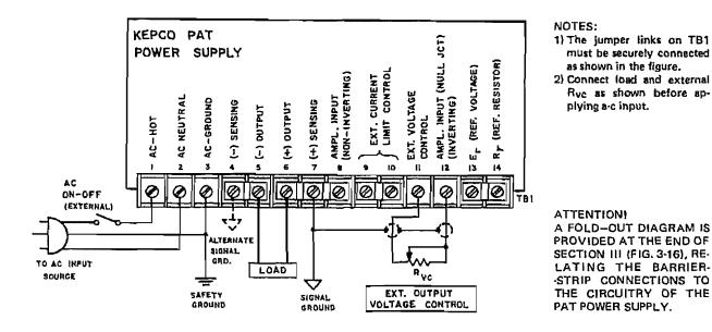
FIG. 2-1 TERMINATIONS AND STANDARD JUMPER-LINK CONNECTIONS.
