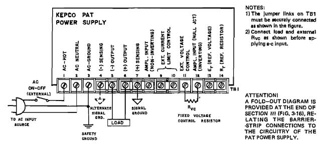
FIG. 3-1 CONNECTIONS FOR FIXED OUTPUT OPERATION.
