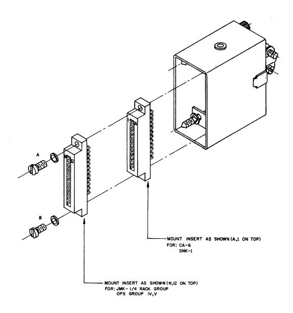
FIG. 1 INSTALLATION OF THE PC-4 MATING CONNECTOR.
